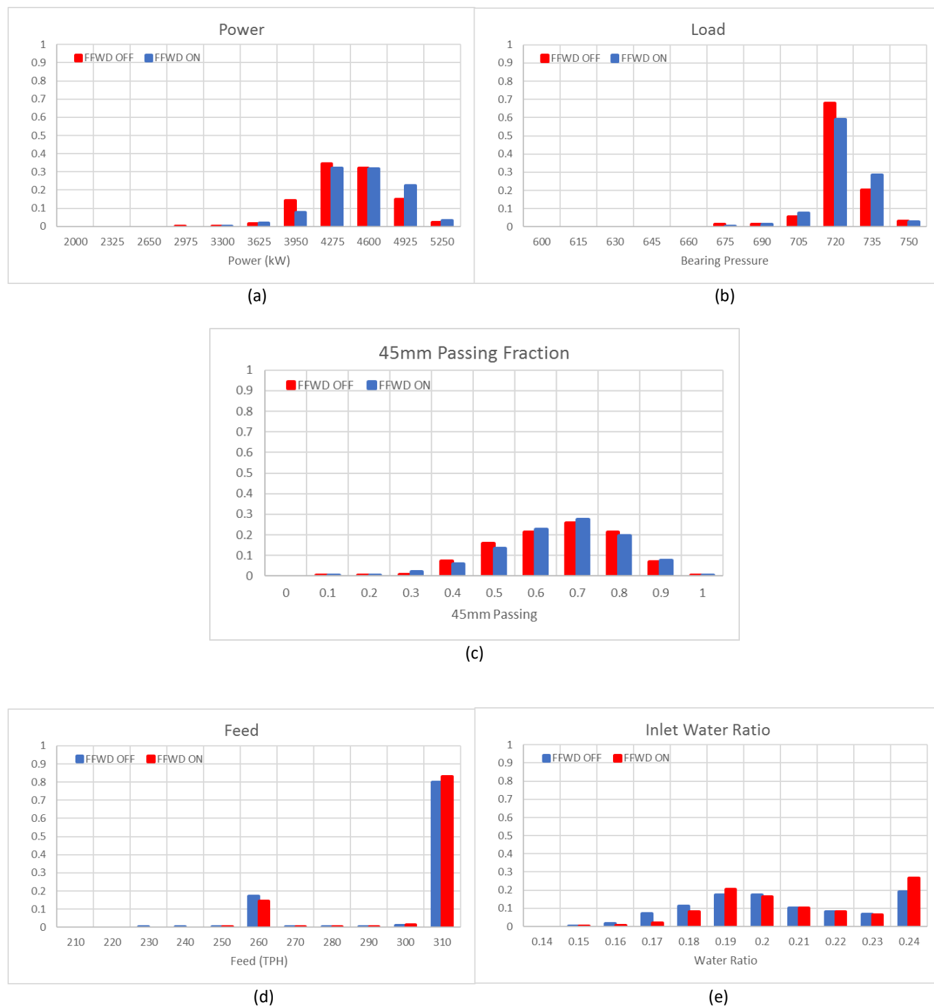
Figure 21: Histograms of the relevant control variables at Mototolo. (a) Power, (b) load, the disturbance signal (c) 45mm passing, (d) feedrate and (e) inlet ratio
